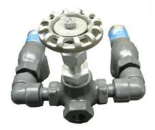
**DUAL ASSEMBLY WITH UNIONS (DU):** Includes two (2) relief valves, one (1) three-way manifold shut-off valve, four (4) 90° elbows, four (4) unions, one "tee" and twelve (12) nipples. (Assemblies using 800, 800SS, 801, 801SS, 800QR, or 803QC valves have only ten (10) nipples.) Only one side of the three-way valve can be closed at any time. This assembly will allow either valve to be changed without disturbing the piping.
